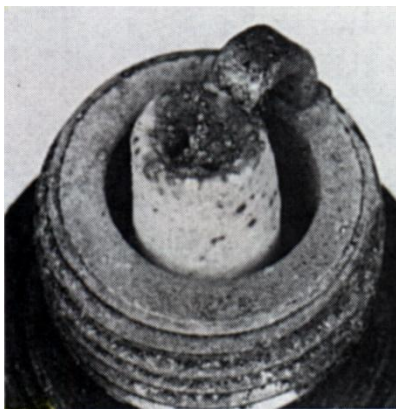
Damage, "salt & pepper" deposits
