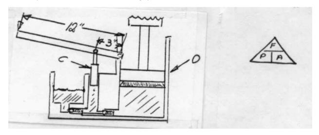
14. If I apply 1 pound of force to the lever in the diagram, how much force is applied to the piston? (tip: The applying force is 12" away from the pivot, the receiving force is 3" away from the pivot.)
