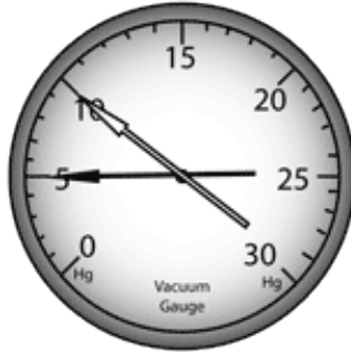
Leaking Intake Manifold Steady Low 5-10 Hg
