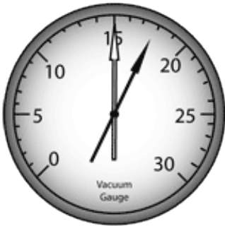
Check Ignition Timing Steady Low 15-18 Hg
