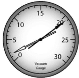
Clogged Exhaust Needle Drops While Accelerating
