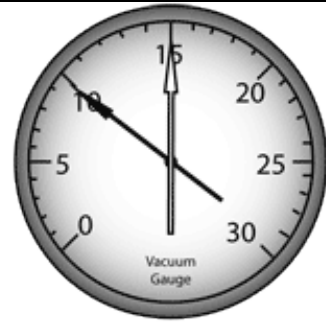
Check Valve Timing Steady Low 10-15 Hg
