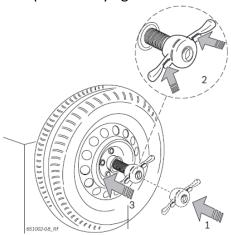
Release the lock and turn the quick-action clamping nut clockwise until the wheel is FIRMLY braced.
