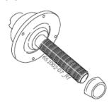
Push the unlocked quick-action clamping nut onto the shaft and press firmly against the wheel
