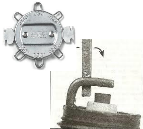
36.5b To change the gap, bend the side electrode only, as indicated by the arrows, and be very careful not to crack or chip the porcelain insulator surrounding the center electrode
