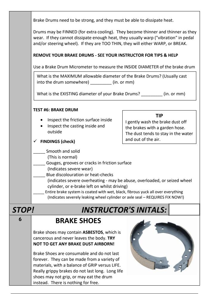
Brake Shoes are usually worn out when the friction material is about as thick as the plate it is glued or riveted to.
