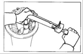
Coat lead paint on 3 or 4 teeth of the ring gear at 3 different locations
