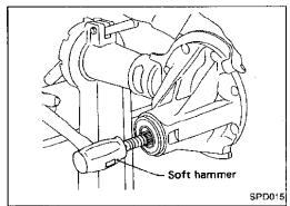
DO NOT remove the bearings unless you have been instructed to do so
