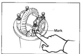
Tighten the bearing cap bolts until the spring washers are slightly compressed.
