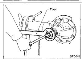
Tighten pinion nut by degrees to the specified preload while checking preload with Tools
