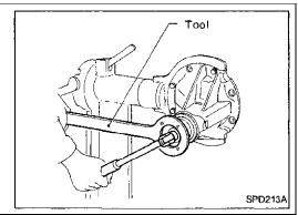
Remove drive pinion with a soft hammer
