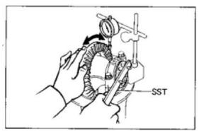
Torque the bearing cap bolts to spec
