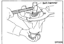
Temporarily tighten pinion nut until there is NO axial play
