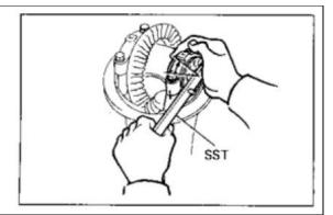
Using a dial indicator, adjust the ring gear backlash to within specification
