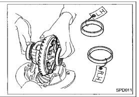
Align marks on the cap and carrier
