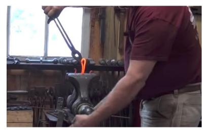
Squeeze the two legs together a bit tighter towards the loop with a BIG pair of pliers
