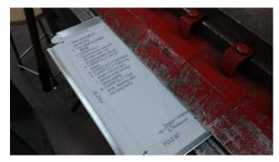
Metal is a little springy (springs are made from it, eh?!), so you have to bend it just a tick further than its "range of elasticity" so it will sit at 90°
