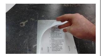
Center punch ALL marked holes with a hammer and a center punch.
