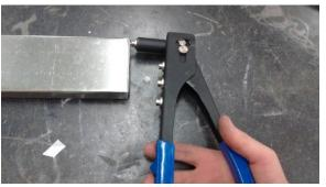
The skinny stick of the rivet has a fat ball on the end. Pulling the stick tries to pull the ball through the fat end. This distorts the fat end so it won't come back out the hole. Ask for a demo on how rivets work!
