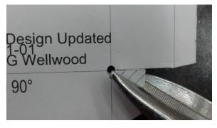
Cut INTO the hole – have the snips END their cut IN the hole (don't over-cut!!)
