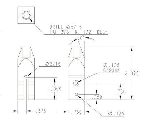
• Still using a FOUR-JAW CHUCK, drill the hole in the end (use a center drill, and then a pilot hole before drilling final size).
