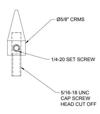
I MADE REMOVEABLE TIPS, AND TURNED A COUPLE DIFFERENT SHAPES. I LIKE HAVING OPTIONS AND/OR THE ABILITY TO MAKE CHANGES.
