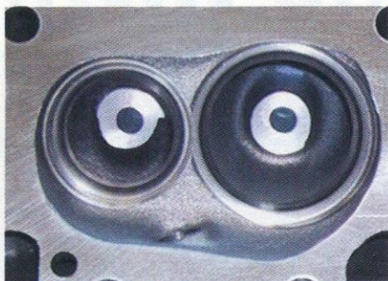
Above: Before and after shots show how blending the valve seats into the guide bowl as well as streamlining the guide bosses can make worthwhile gains.
